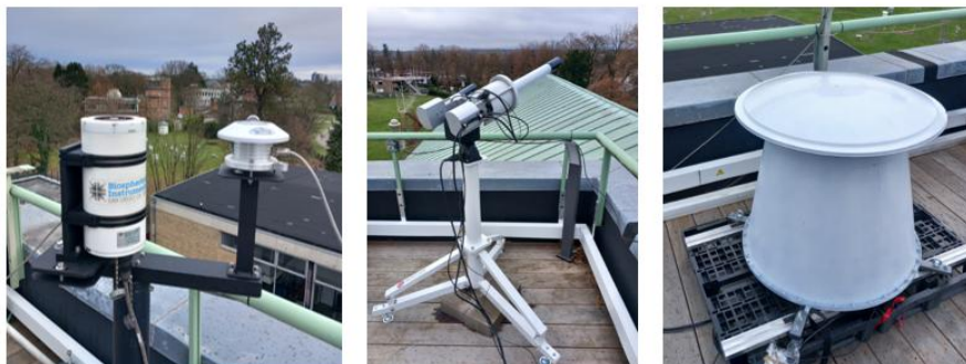
Figure 3.17: Left: UVB pyranometer (model MS-212W from EKO) and multi-channel radiometer (GUV-2511 from Biospherical), installed on the roof of BIRA-IASB. Center: Gigahertz Optik BTS2048-UV for AOD and TOC measurements. Right: neutron detector from BFKH (Hungary).
