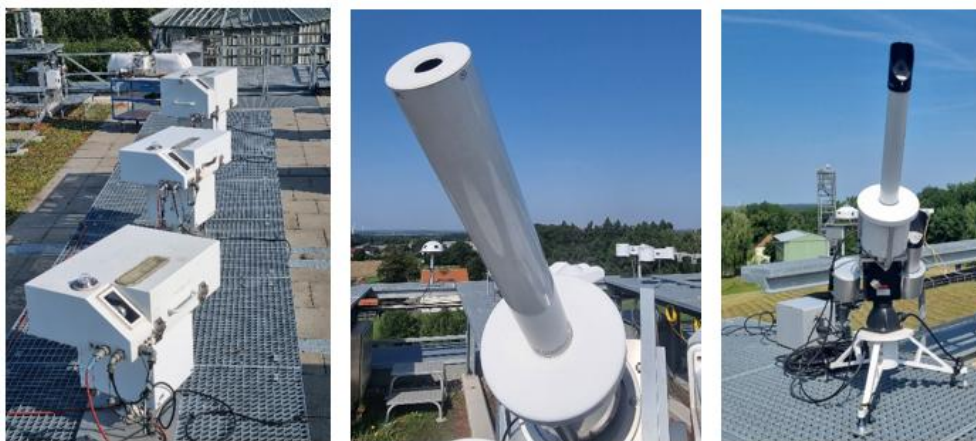
Figure 3.40: TOC (Total Ozone Column) instrumental suite of the DWD Lindenberg Campaign on the rooftop of MOL-RAO ‘SMZ’ building. Left: DWD instruments Brewers and Dobson (background). Middle: DWD BTS2048-UV in direct-sun mode. Right: Gigahertz-Optik BTS2048-UV in direct-sun mode.
