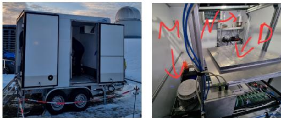
Figure 3.39: Secondary Cosmic Rays (SCR) instrumental suite of the DWD Lindenberg Campaign in the PTB trailer (left) at MOL-RAO. Inside the trailer (right): PTB muon detectors MUDOS (“M”) and DECOS-2 (“D”), and the UJF-NPI neutron detector (“N”). Not shown in the picture, but also present in the trailer during the campaign, were ADVACAM Timepix micro-telescopes.
