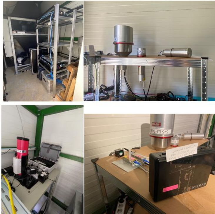
Figure 3.28: PTB muon detector and UJF SEVAN detector, UJF neutron detector, UJF gamma-ray spectrometer RT-56, ADVACAM Timepix3 SCR particle tracker detectors
