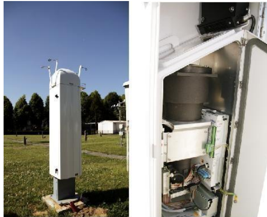
Figure 3.16: Automatic LIDAR Ceilometer measuring the backscattering signal by aerosols, fog and clouds.
