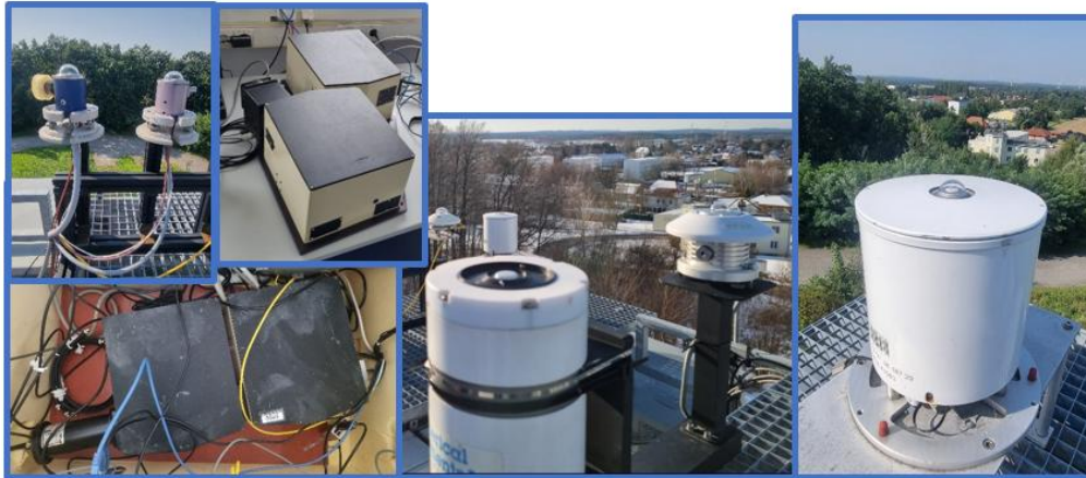
Figure 3.41: UV instrumental suite of the DWD Lindenberg Campaign on the rooftop and in the MOL-RAO ‘SMZ’ building. Left: DWD Bentham DTM 300 (below) and BIRA-IASB Bentham DTM 300 (above right), with their optical entrance on the roof (above left). Middle: BIRA-IASB GUV-511 multi-filter radiometer (left) and UV-Pyranometer (right). Right: DWD BTS2048-UV in global measurement mode.
