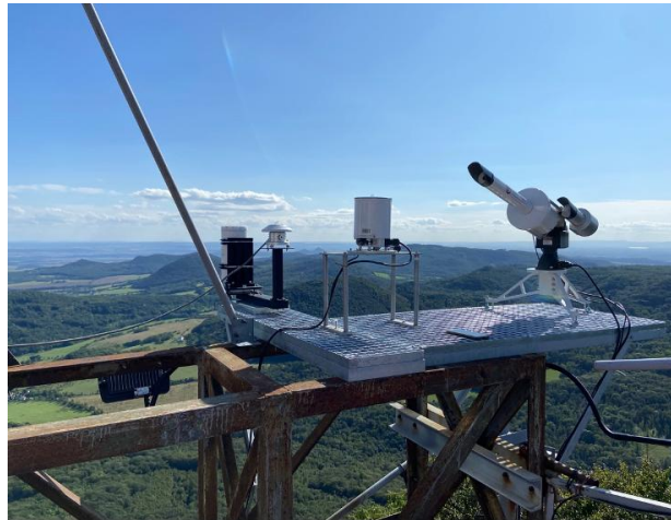
Figure 3.29: The UV-Index and TOC suite: from left to right: BIRA-IASB GUV and UV pyranometer DWD BTS, GHO BTS-direct, on the rooftop platform of Milešovka observatory.
