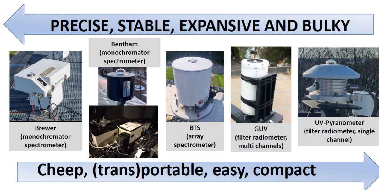
Figure 2.6: UV instruments deployed in the BIOSPHERE campaigns, ranging from precise but bulky and labour-intensive (left) to modern, portable, and easy-to-use (right).
