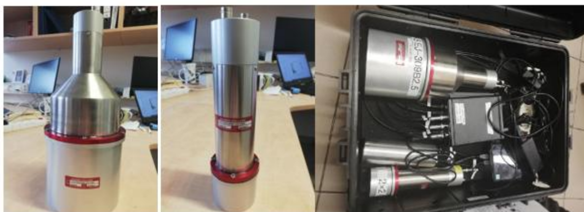
Figure 2.2: Neutron detector – large scintillator 5x5" (left), small scintillator 2x2" (center), and box with all components (right).
