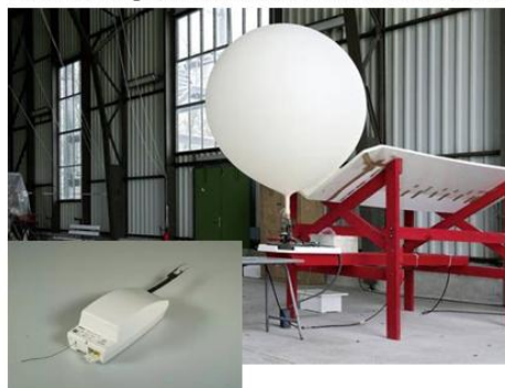
Radiosounding with Vaisala RS41 and weather balloons
