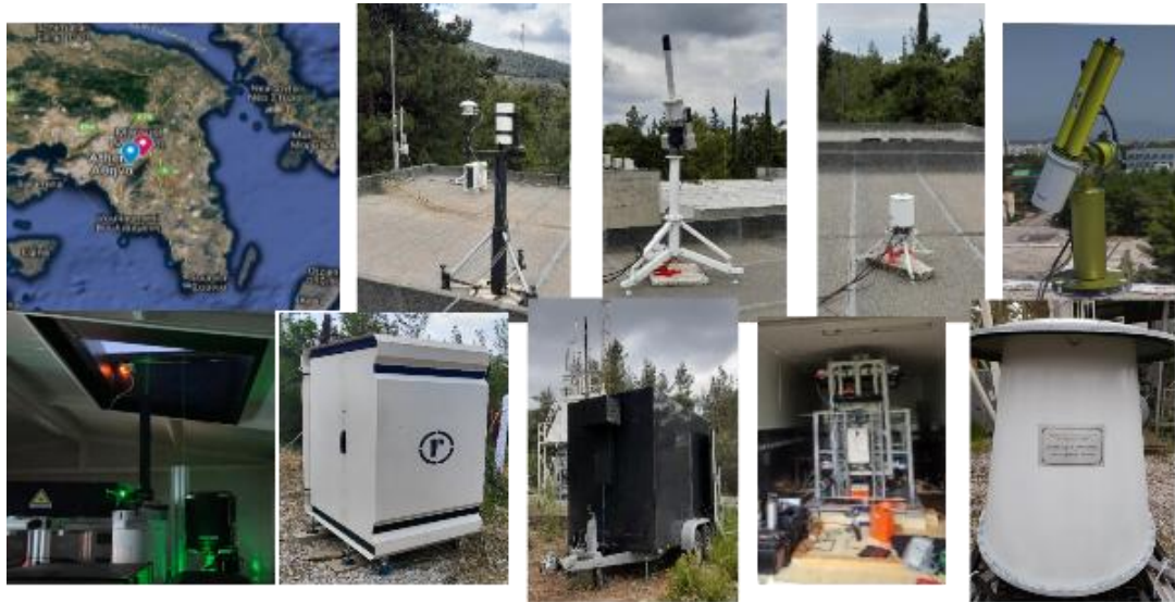
Figure 3.1: (upper left to down right) NCSR-DEM and NTUA sites, UV spectroradiometer, BTS solar sun tracker, UVB pyranometer, GUV-511 multi-filter radiometer, NTUA and Raymetrics lidars, neutron, muon detectors.
