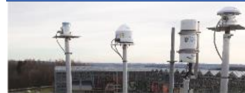
BIRA-IASB: UVB pyranometer and GUV-511 multichannel filters radiometer
